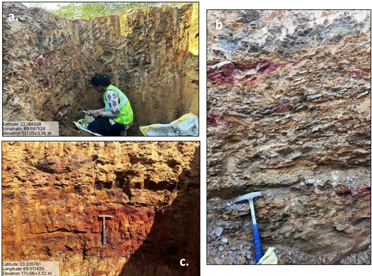
Fig. 6.3 Representative pit exposures showing lithological variations across the Katrol and Bhuj Formations in the Bhuj exploration block. (a) Pit exposure within the Katrol Formation showing shale-dominated heterolithic sequence with alternating layers of shale, siltstone, and tuffite interlayers. Note the gradational contacts and ferruginous staining along bedding planes. (b) Close-up view of the heterolithic succession displaying thin, lenticular ferruginous tuffitic laminae at multiple levels. (c) Pit exposure within the Bhuj Formation showing medium- to fine grained ferruginous sandstone with variable degree of Fe-oxide impregnation. Note the transition between the metasomatized ferruginized sandstone and the ferruginized sandstone at the top part of the pit wall.
