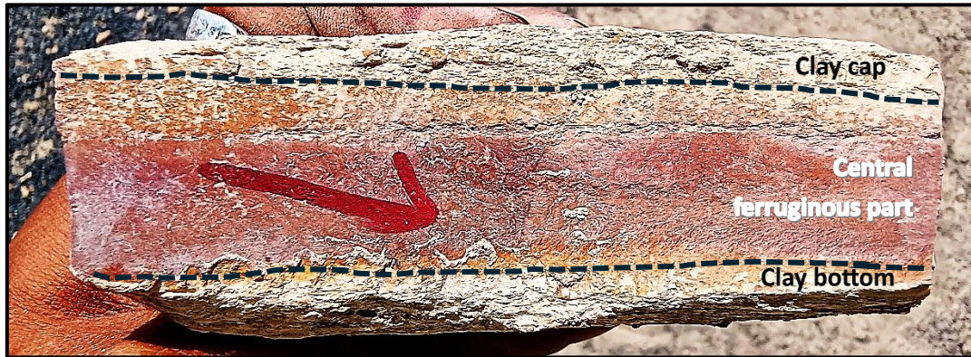
Fig. 4. 24 Hand specimen of a tuffite layer from the Katrol Formation showing distinct bedding-parallel compositional banding and tripartite layering.
