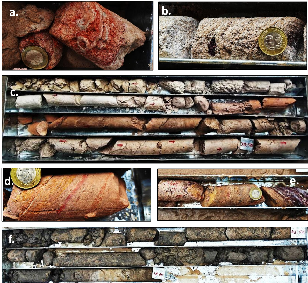
Fig. 6. 15 Megascopic photographs of core sections from Borehole GSPL_Bhuj_BH-04, showing representative sedimentary unit. (a) Sandstone with differential ferruginization at 18 m (b) Lense shaped Iron solution (Hematite) in ferruginous Sandstone at a depth of 32.20m (c) Shale Sandstone Hetrolith at 33.50 to 37.60 m (d) Alteration of Shale (alternative layer of hematite and goethite) at 35. 46m (e) Mica bearing metasomatized sandstone at 44.10 to 44.50 (f) Breccia unit at 45.50 to 48 m.
