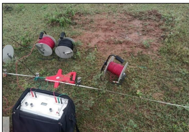
Fig. 4. 58 (a) Aquameter CRM 500 used to Collect the Resistance Data. (b) Basic Concept of Resistivity Measurement.
