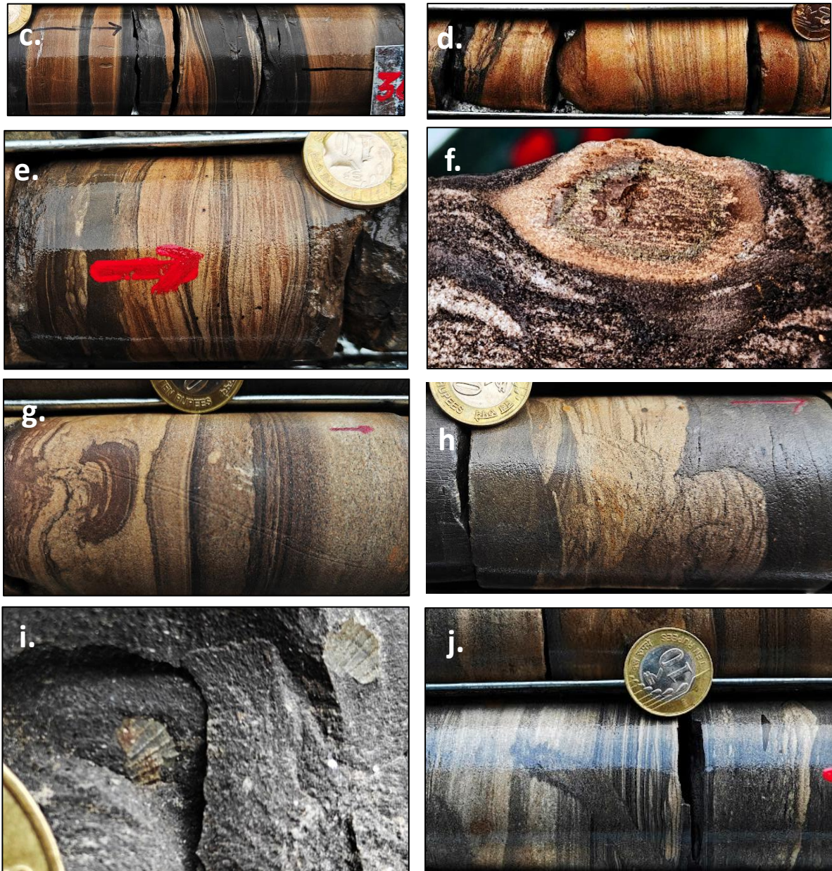
Fig. 6. 6 Megascopic photographs of core sections from Borehole GSPL_Bhuj_BH-01, showing representative sedimentary structures within the shale-dominated heterolithic unit. (a) Wavy to plane-parallel lamination with intercalated tuffitic lenses and lapilli-sized volcanic fragments. (b) Flaser, lenticular, and wavy bedding. (c) Suspected tuffite layers. (d) Bouma sequence. (e) Hummocky cross-stratification and ball-and-pillow structures. (f) Sand layers with disseminated pyrite/chalcopyrite within shale-dominated heterolith. (g) Soft-sediment deformation with wavy parallel lamination and iron leaching. (h) Load casts and flaser bedding within shale of shale-sandstone heterolith. (i) Occurrence of bivalve fossil. (j) Trace fossil and burrow with soft-sediment deformation, flaser bedding, and lapilli-bearing layer.
